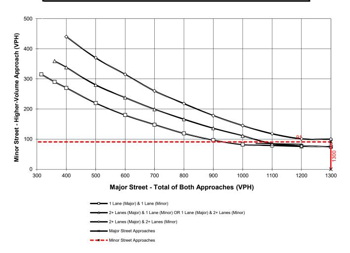
\*Note: 100 vph applies as the lower threshold for a minor-street approach with two or more lanes and 75 vph applies as the lower threshold for a minor-street approach with one lane
