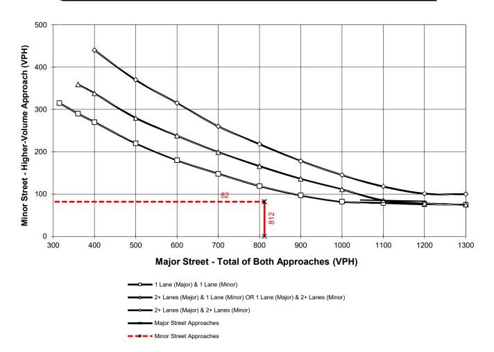
\*Note: 100 vph applies as the lower threshold for a minor-street approach with two or more lanes and 75 vph applies as the lower threshold for a minor-street approach with one lane
