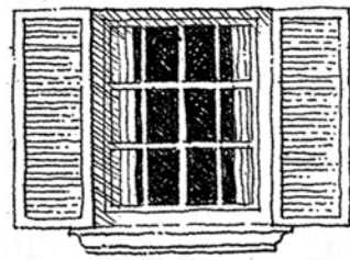
WINDOW WITH LOUVERED SHUTTERS
