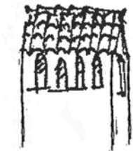
STUCCO AND TILE ARCH OPENING AT GABLE & SIDE OPENING
