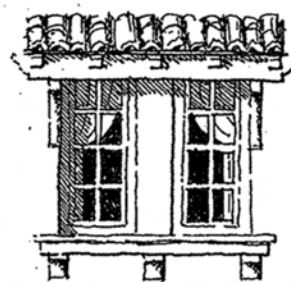
PAIRED WINDOW WITH CORBELED ROOF AND BRACKETS
