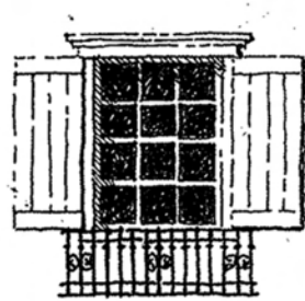
WINDOW WITH DECORATIVE WROUGHT IRON RAILING
