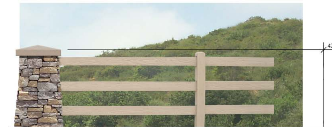
Option #4 Description: -Three Rail Vinyl Theme Fence -CMU Pilaster with Decorative Stone Veneer and Concrete Cap
