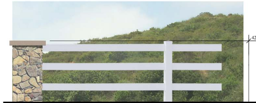
Option #1 Description: -Triple Rail Vinyl Theme Fence -White, Tan or Black Integral Color -CMU Pilaster with Field Stone Veneer and Concrete Cap
