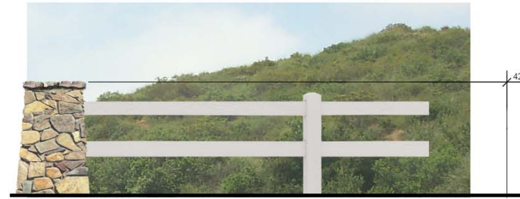
Option #2 Description: -Double Rail Vinyl Theme Fence -White, Tan or Black Integral Color -CMU Pilaster with Field Stone Veneer and Field Stone Cap
