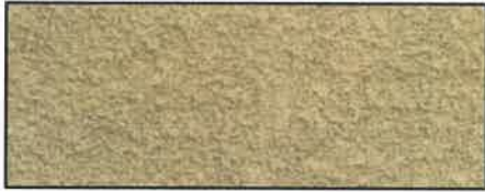
STUCCO: 7/8" CEMENT PLASTER TEXTURE: (FINE SAND FINISH)
