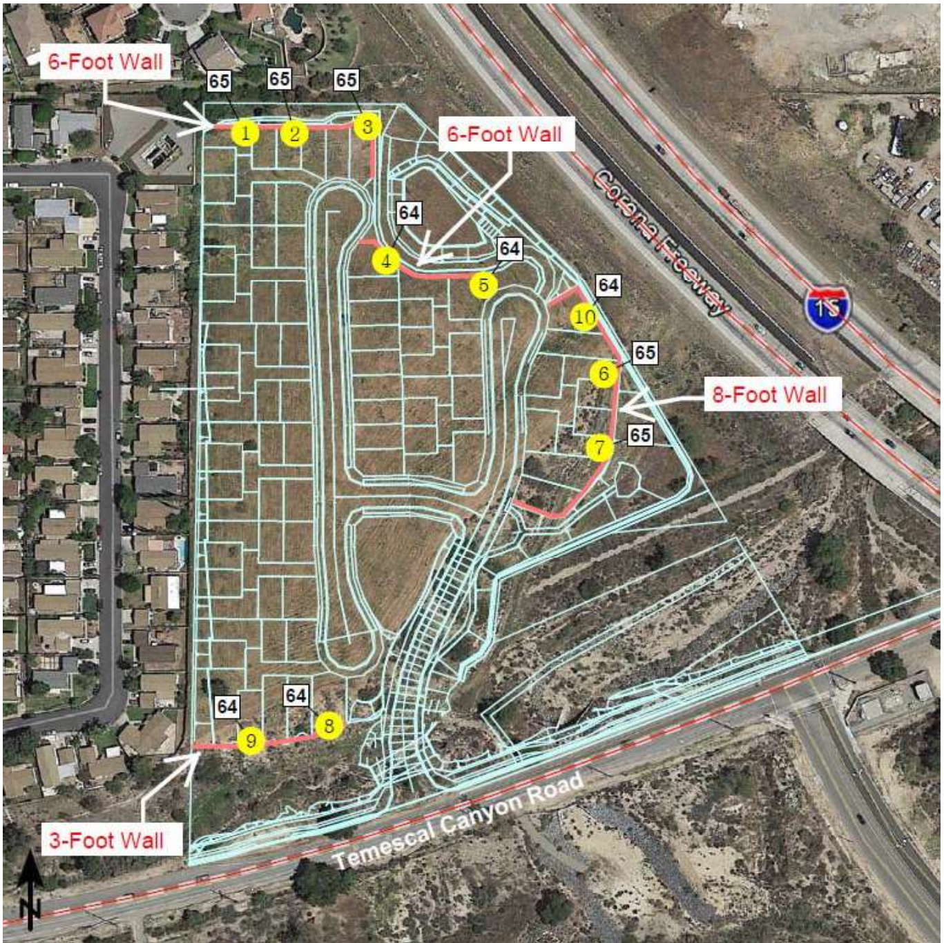
Figure 32-2 Mitigated Traffic Noise Levels (CNEL)
