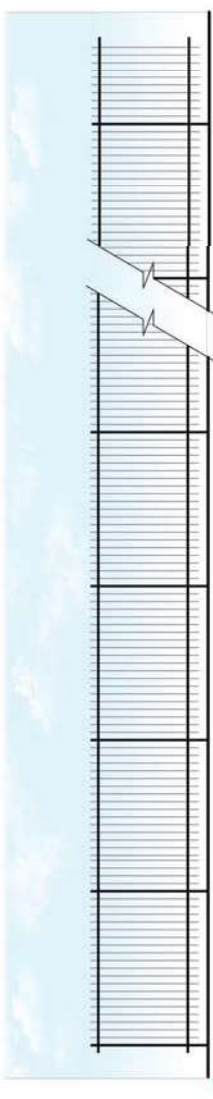
3 OPEN VIEW FENCE | 6' TUBULAR STEEL FENCE MAINTAINED AS NOTED ON PLAN N.T.S.
