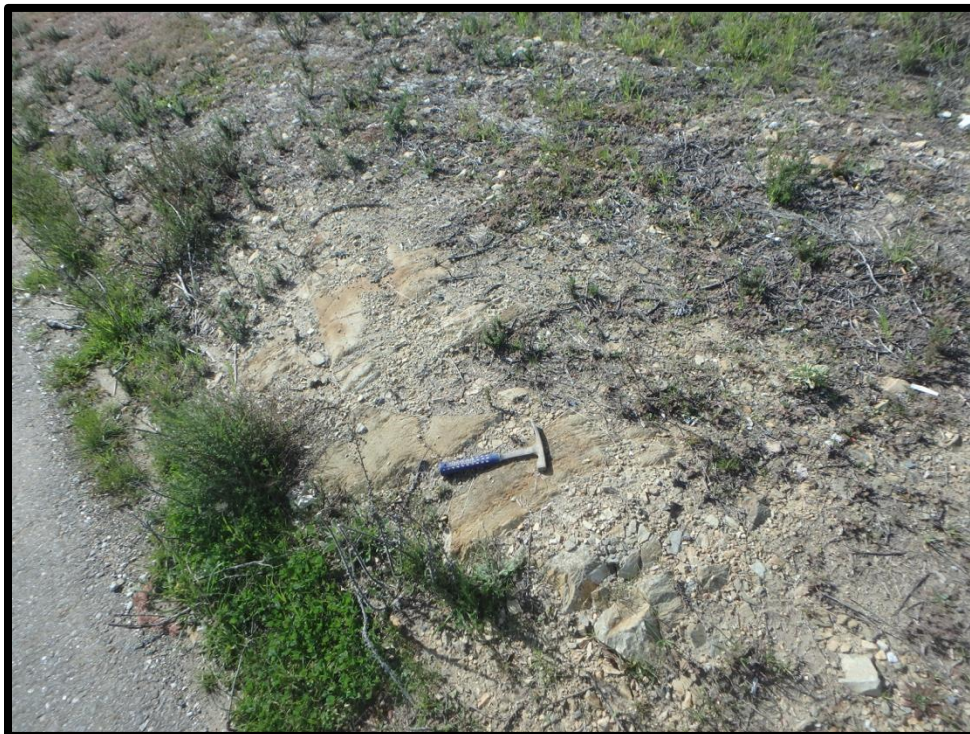
Figure 17. Metamorphic grade bedrock exposed in a rock cut along SR-79 adjacent to the southeastern corner of the survey site. Mapped as Pleistocene-age alluvium (Qvova) and Mesozoic phyllite (Mzp). View down.
