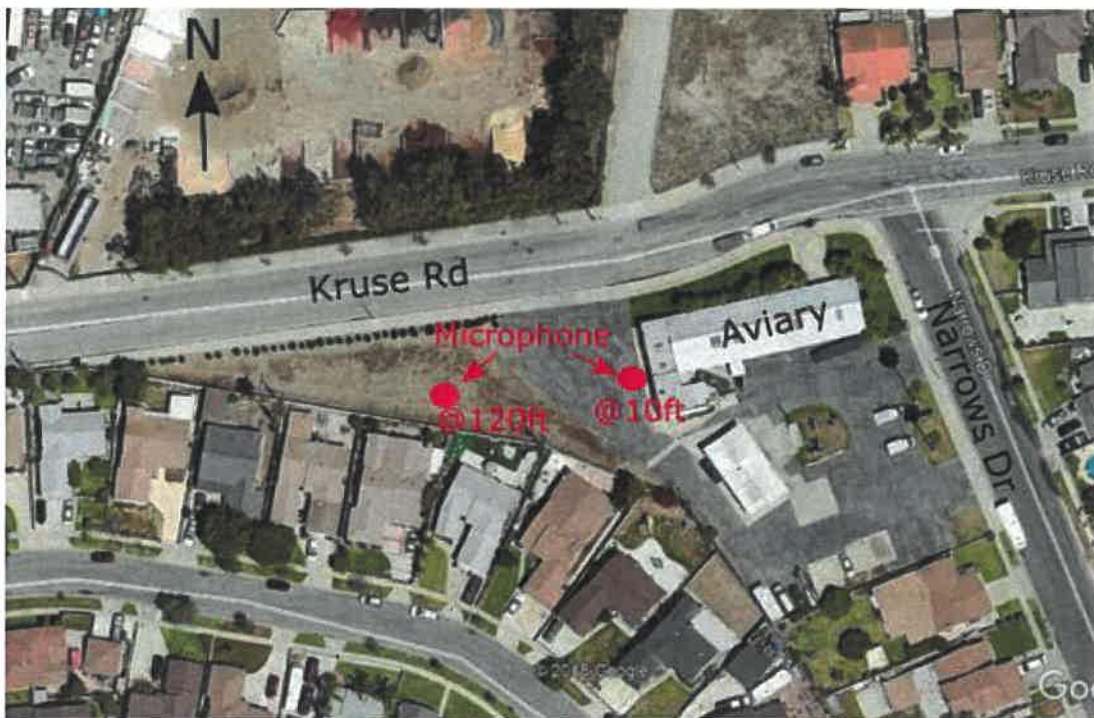
Figure 1: Aerial photograph showing the location of microphones during noise measurement
