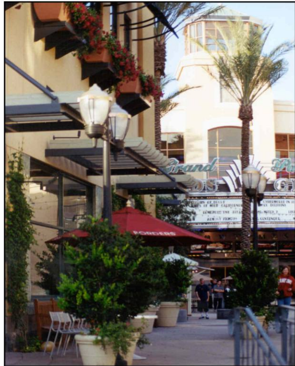
Note variations in building facade treatment including awnings, trellises structures, pilasters, and display windows.
