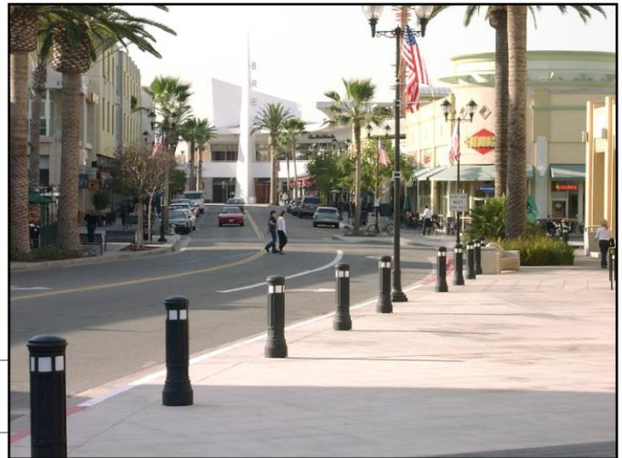
These bollards not only serve as a deterrent for vehicular traffic; they also provide an opportunity to create attractive lighting elements.
