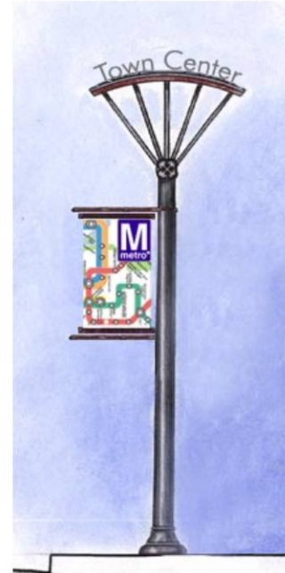
This sign has a dual purpose: it serves as a neighborhood identifier and transit stop sign. Combining signs minimizes the amount of sidewalk space used for uses other than pedestrian traffic flow.
