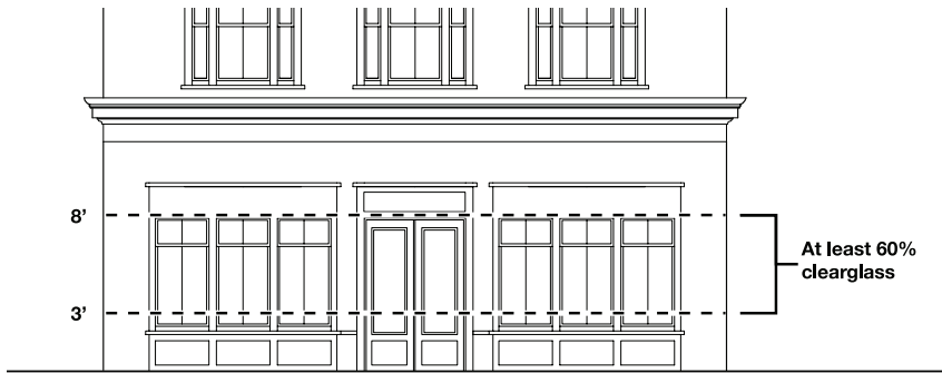
Figure 3. Ground-level retail and service uses with minimum amounts of clear glass façades
