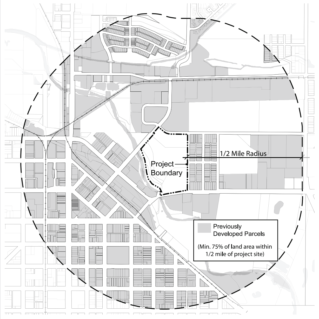
(c). Infill project site based on minimum 75% of land area within 1/2 mile of project boundary being previously developed
