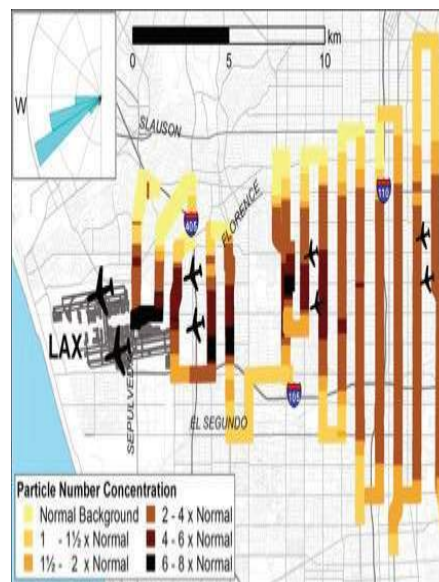
Graphic depicting ultrafine particle increase downwind of LAX relative to urban background air quality (Graphic/Neelakshi Hudda)
