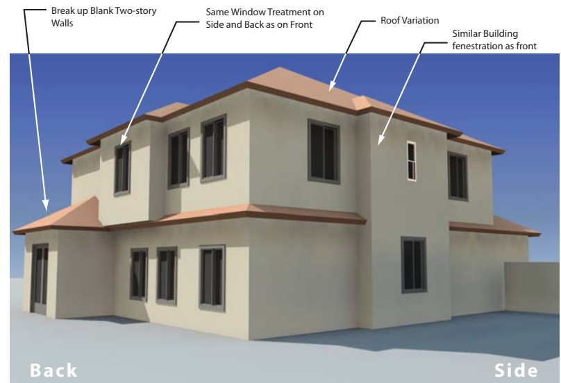
Exhibit 70 | Two-Story Back & Side - Acceptable
