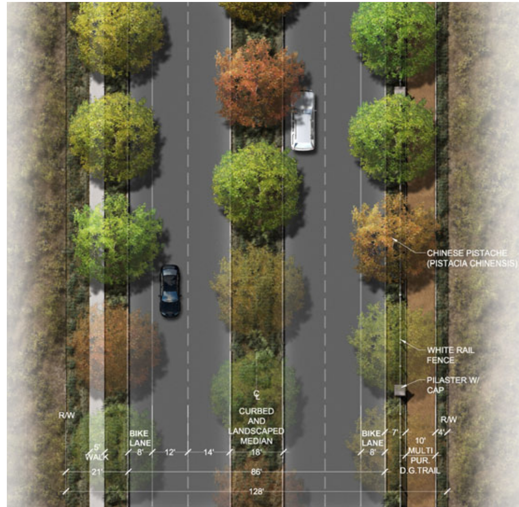
Exhibit 46 | Road A - Typical Temescal Canyon Road Plan Temescal Canyon Road’s many amenities will include a multi-use trail, landscaped median, and parkway sidewalk. Chinese Pistache trees will provide dense green canopies in the summer and dramatic color in the fall. North is up on drawing.
