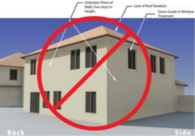
Exhibit 22 | Two-Story Back & Side - Unacceptable
