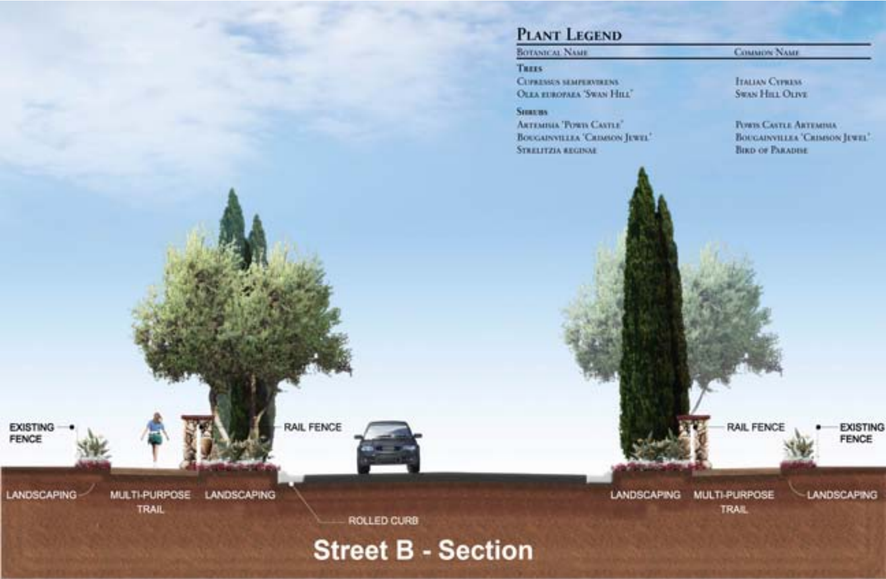
Nuevo Road section - The landscape palette will feature the vertical relief of odd-numbered clusters of Italian Cypress placed among the broad canopy of olive trees. Color accents will be provided by perennial shrubs along the parkway.
