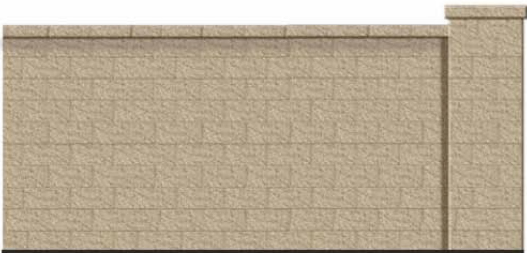
Block Wall & Pilaster Integral Color, Split Face CMU Block Wall (Facing Common Areas) Integral Color CMU Cap With 1" Overhang On Each Wall Face Integral Color Split Face CMU Pilaster Integral Color CMU Pilaster or Pre-cast Concrete Cap (* Color: "La Paz" Manufactured by RCP Block and Brick) (Note: Provide 1 Gal. Parthenocissus Tricuspidata Vines Along All Tract Walls Facing Common Areas at 10' Spacing Typical)
