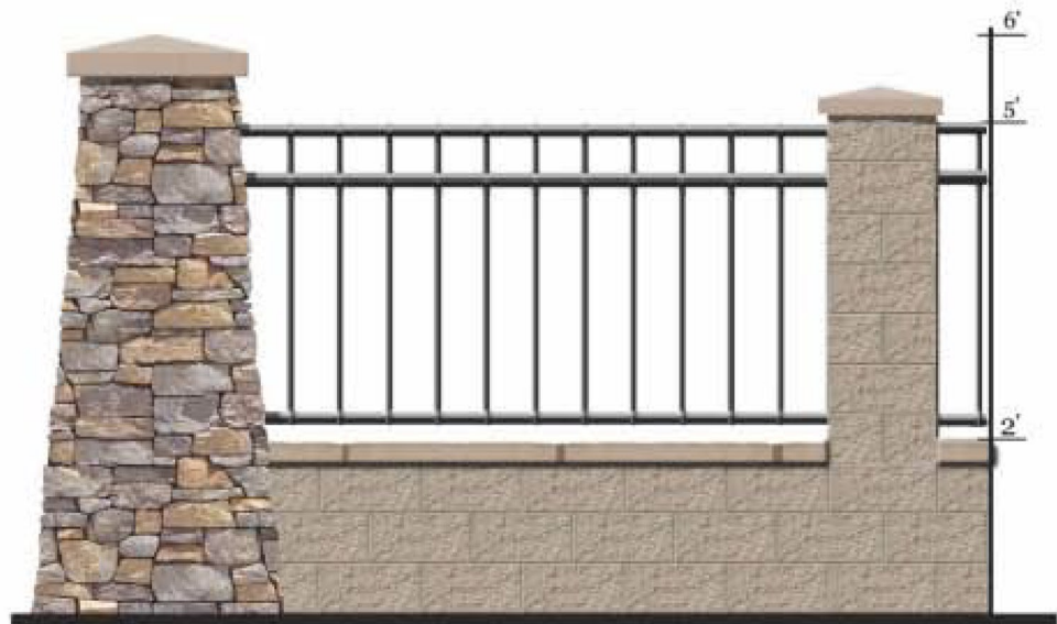
Split Wall/View Fence 2' Split Face Block With Wall Cap 3' Tubular Stainless Steel View Fence Battered Stone Veneer Pilaster With Concrete Cap in Accent Areas
