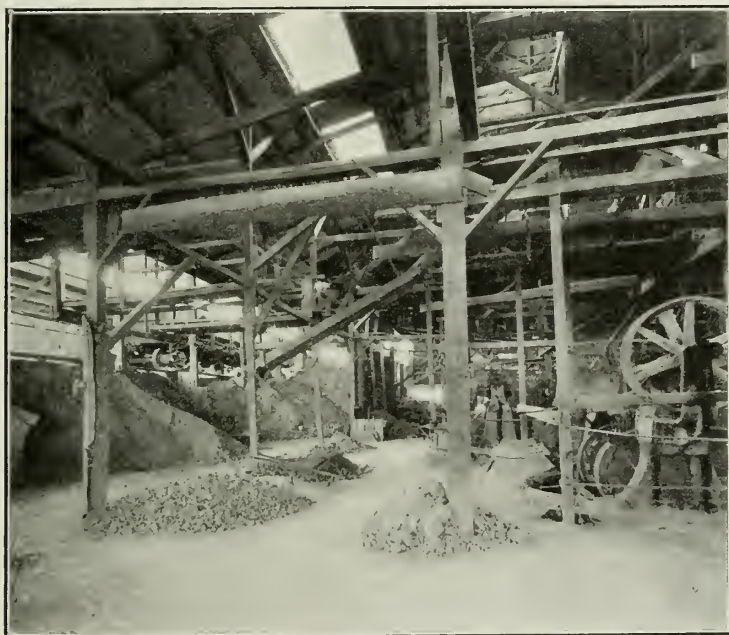
PHOTO No. 64. Clay bins and dry pans in plant of the Stockton Fire Brick Company. (Photo by courtesy of the company.)
