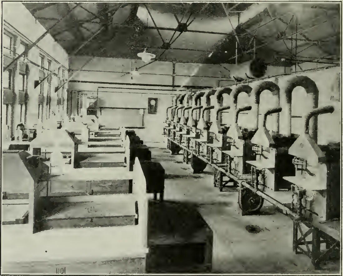
PHOTO No. 67. Assay laboratory, Stanford University, showing muffle furnaces in which test pieces were fired.
