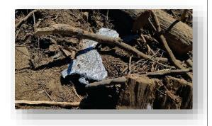
**Figure 4.** This is a view of an ingot or solidified molten metal, possibly resulting from the recent fire. Low melting point and sheen, as well as weight, suggest it may be lead or other similar metal.
