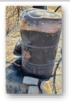
**Figure 7.** This is a view of a distorted 50-gallon drum with leakage at the bottom as evidenced by the stained soil.
