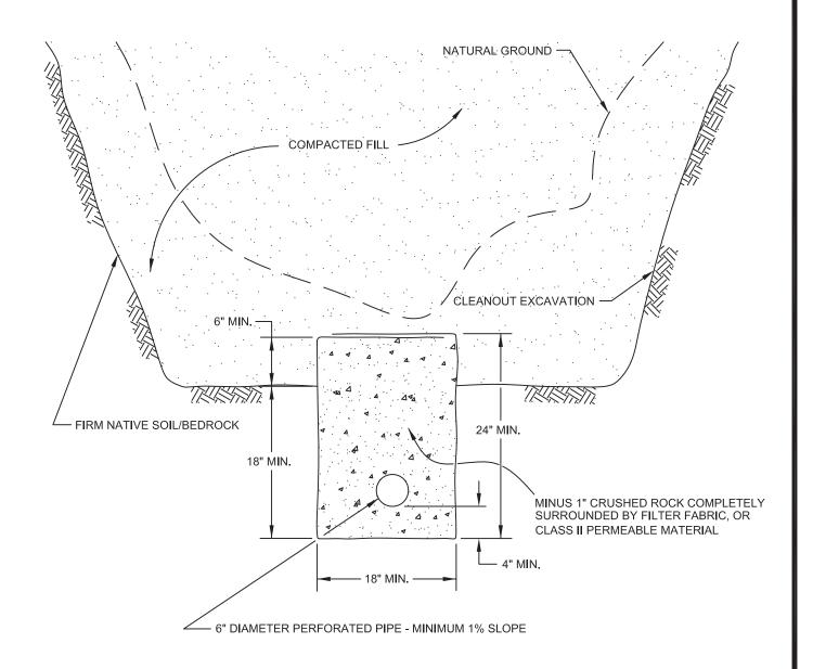
PIPE MATERIAL ADS (CORRUGATED POLETHYLENE) TRANSITE UNDERDRAIN PVC OR ABS: SDR 35 SDR 21
