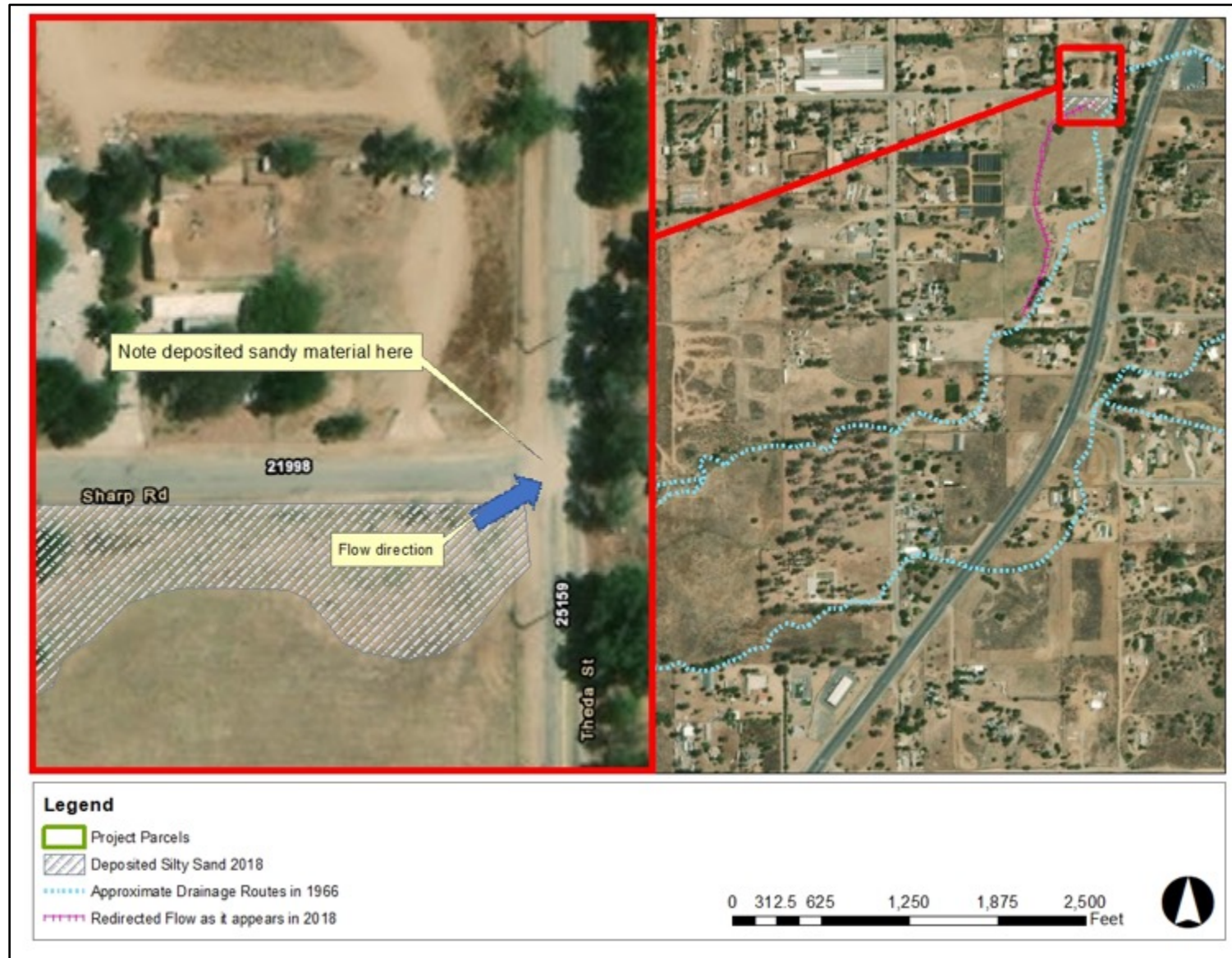
Figure 14. Modified Drainage and Deposited Alluvium from Flooding.
