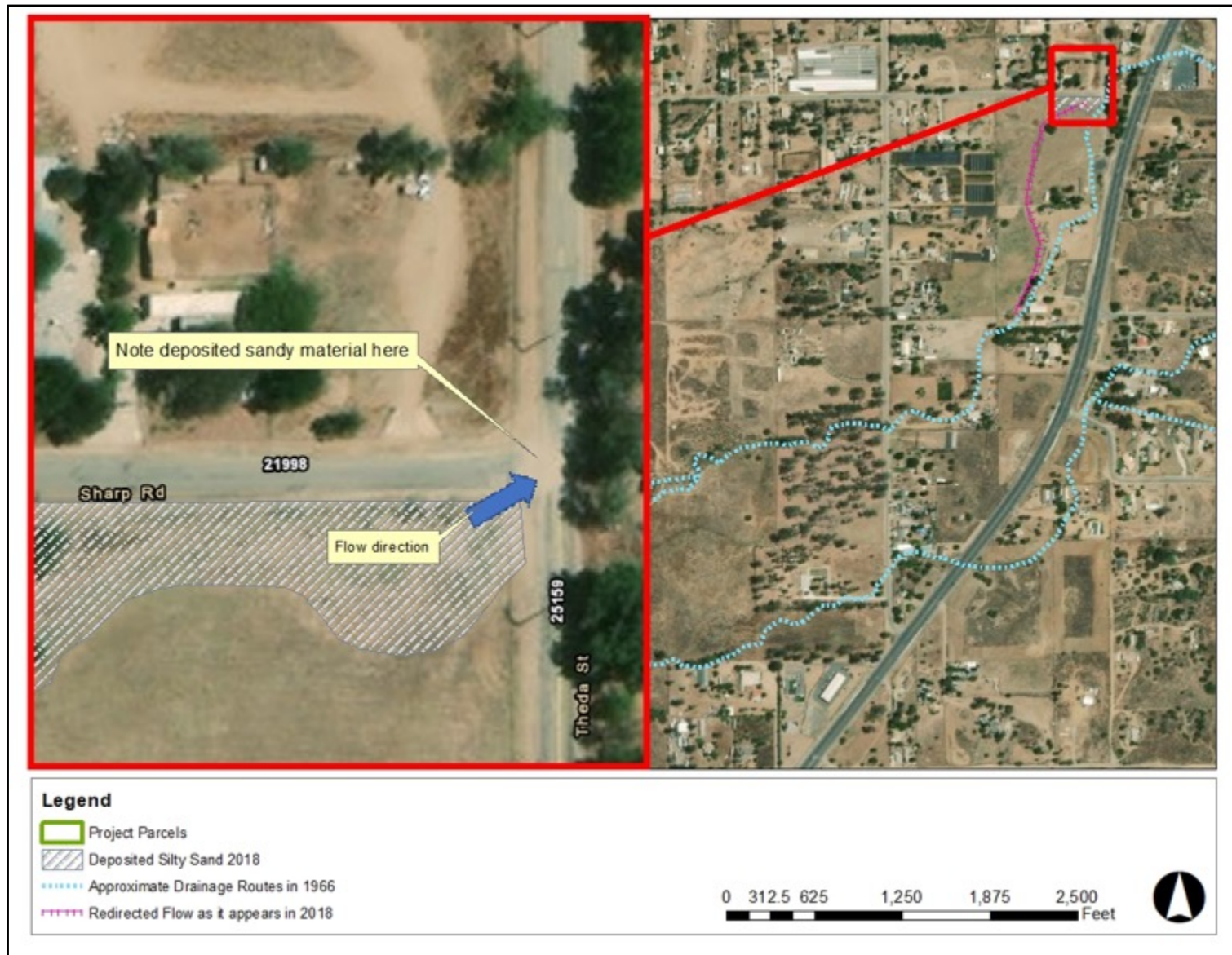
Figure 14. Modified Drainage and Deposited Alluvium from Flooding
