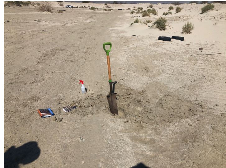
Photo 8. View of WDP 2, facing west, within NWW-2 after the feature transitions to a detention basin. WDP 2 met the wetland hydrology parameter; however, WDP 2 did not meet the hydrophytic vegetation or hydric soil parameters (33.830669, -116.395343). May 25, 2022
