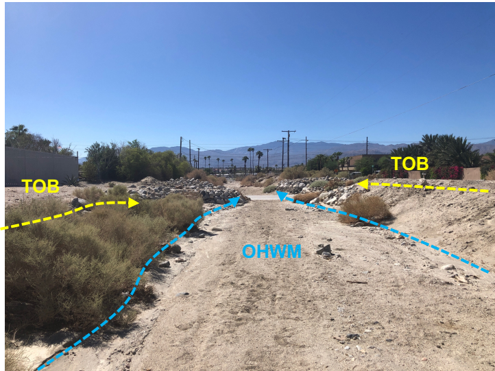
Photo 13. Downstream view of ODP 4 within NWW-3, facing south, within disturbed desert saltbush scrub. ODP 4 exhibited a break in bank slope, change in average sediment texture, change in vegetation species, and change in vegetation cover (33.818154, -116.386089). September 21, 2022.
