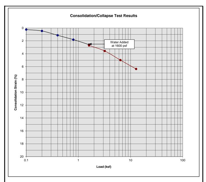
Classification: Light Brown Silty Clay to Clayey Silt, trace fine to coarse Sand
