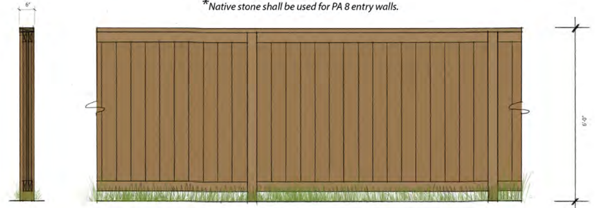
6' SOLID WALL - WOOD OR PVC FENCE
