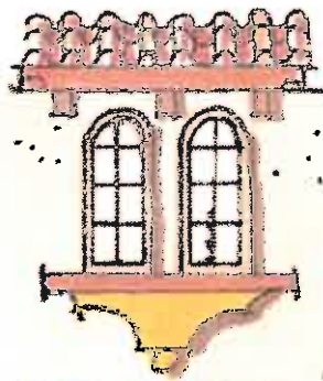
Paired Windows W/ Corbeled Roof And Brackets
