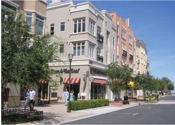
Vertical and horizontal offsets and architectural elements help to create variety in building mass.
