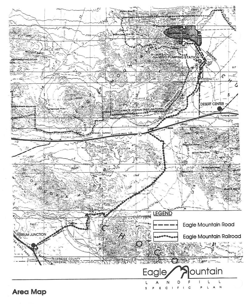
Presently, the Eagle Mountain rail line connects Ferrum Junction with the Eagle Mountain mine. During initial operation of the landfill, this existing rail line will be used in its entirety to access the rail yard in Planning Area 2. When waste volumes warrant, a new 2 mile long rail spur will be constructed, departing from the Eagle Mountain rail line at a point southeast of the existing landing strip and terminating at the rail yard in Planning Area 3.
