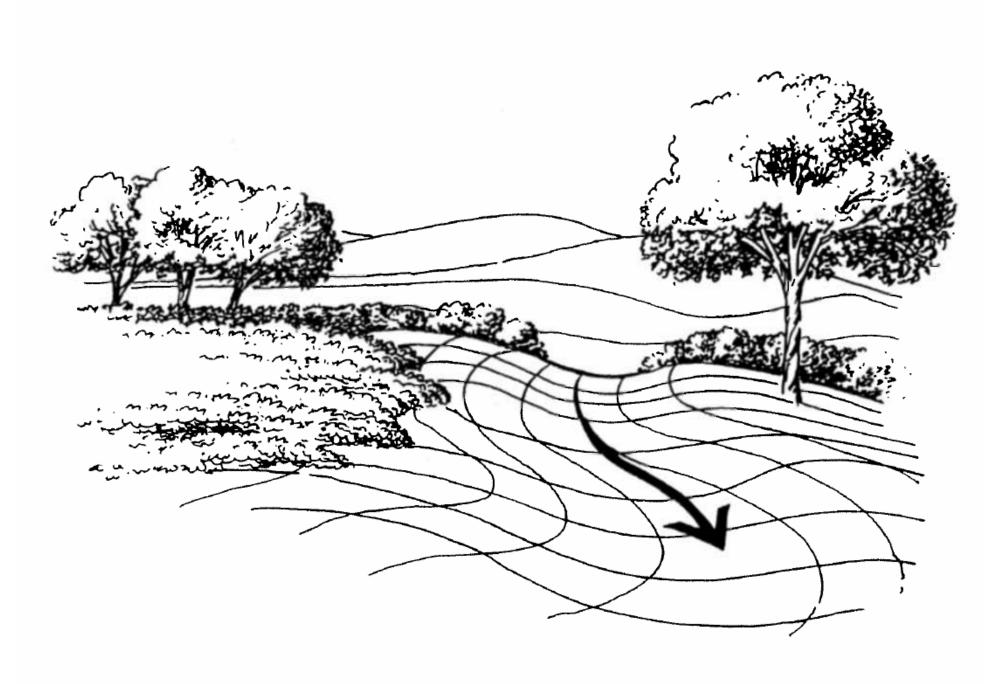
Design drainage swales to use the natural surface runoff for plant irrigation, minimize engineered look.
