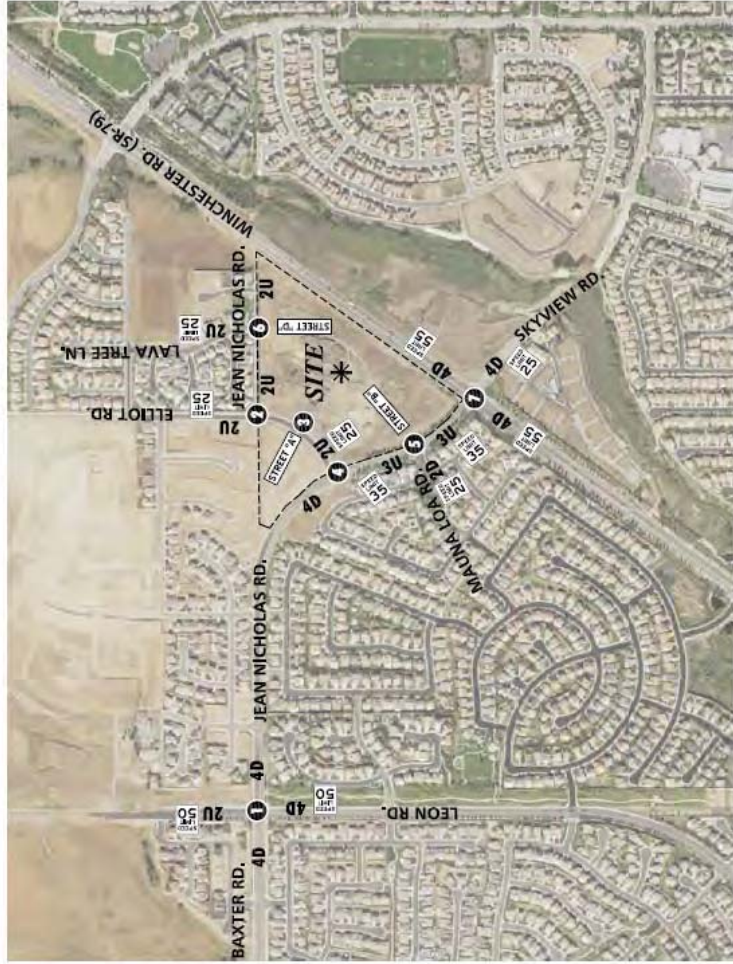
Figure 37-1 Existing Number of Through Travel Lanes and Intersection Controls
