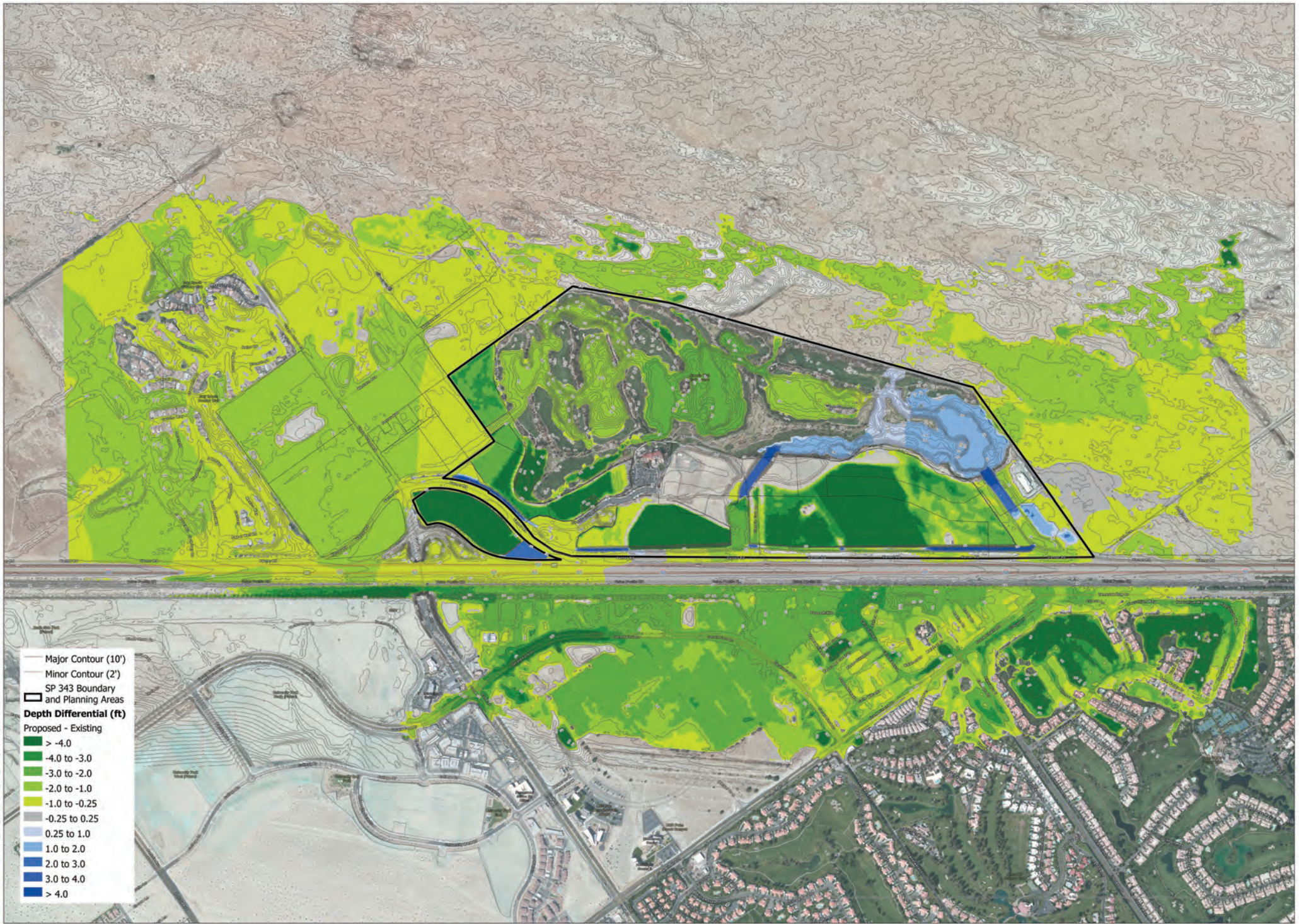
BERGER FOUNDATION Q 100 = 11,600 CFS FLOODPLAIN ROUTING
