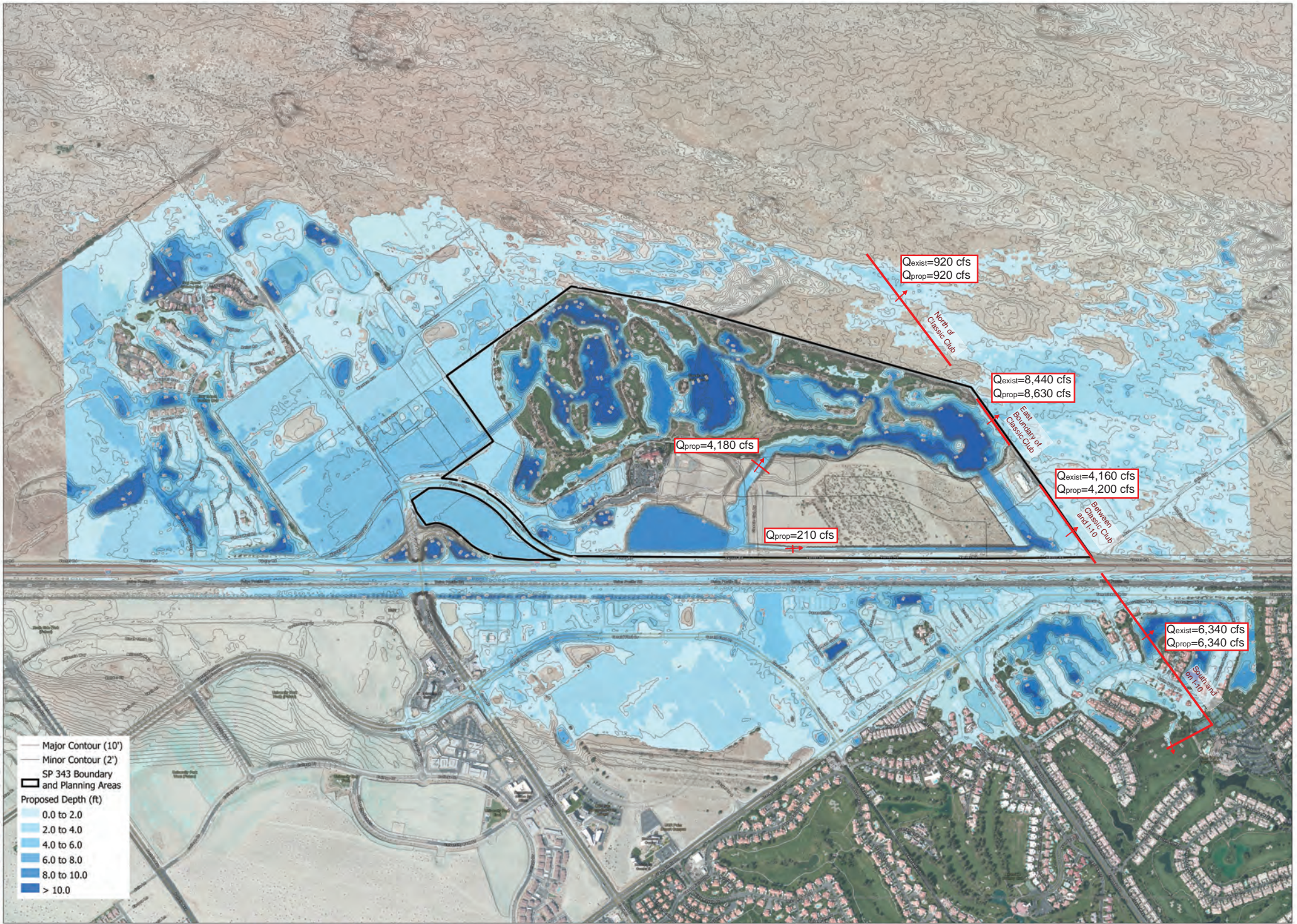
BERGER FOUNDATION Q^{100} = 26,360 CFS FLOODPLAIN ROUTING
