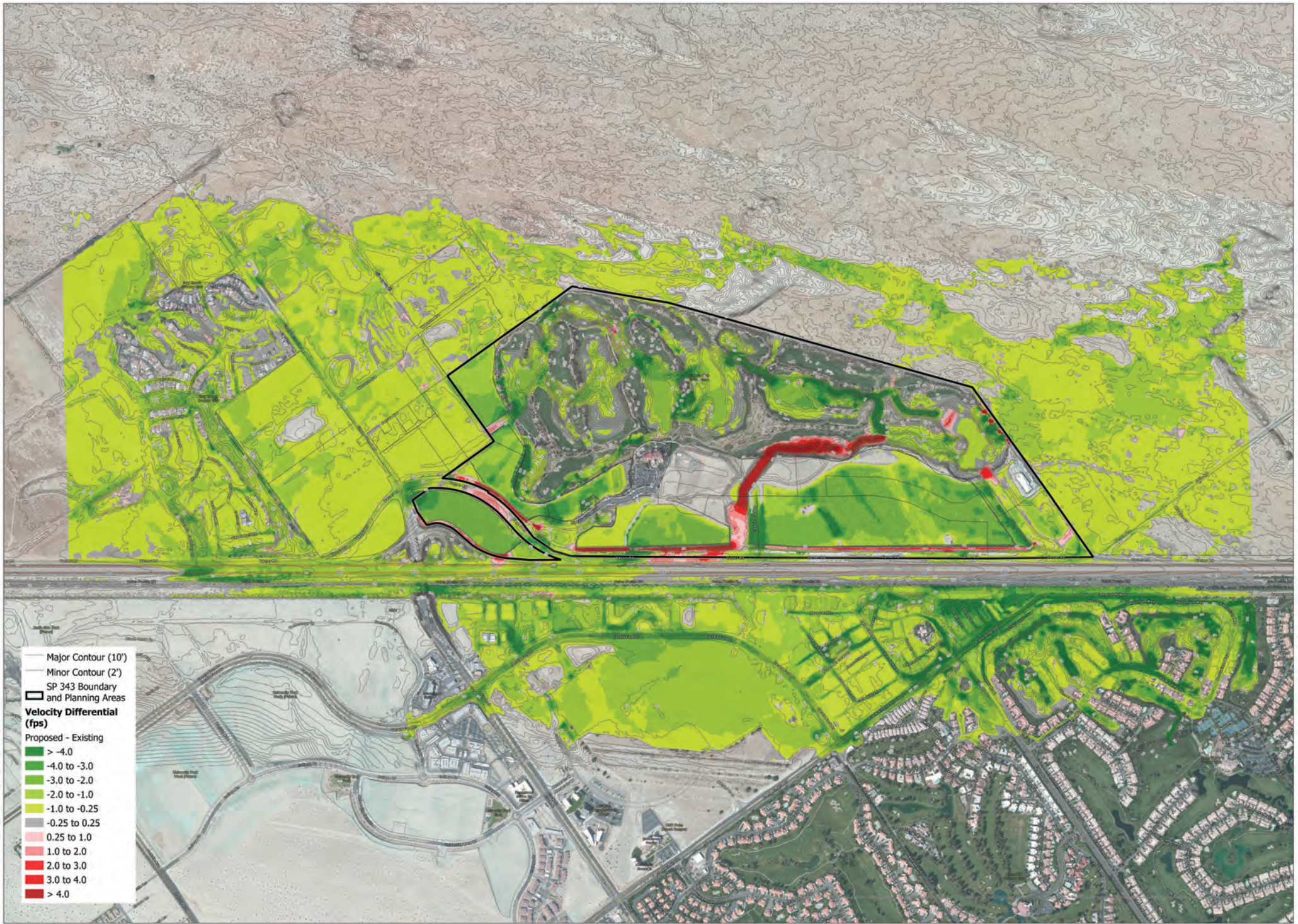
BERGER FOUNDATION Q 100 = 11,600 CFS FLOODPLAIN ROUTING
