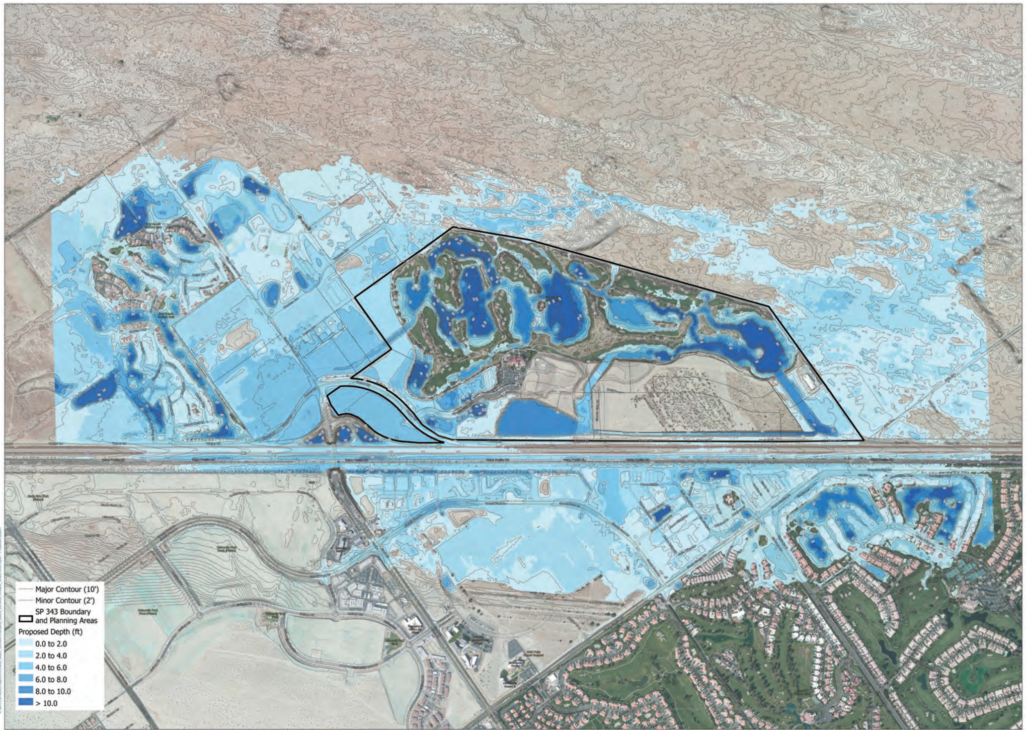
BERGER FOUNDATION Q 100 = 26,360 CFS FLOODPLAIN ROUTING
