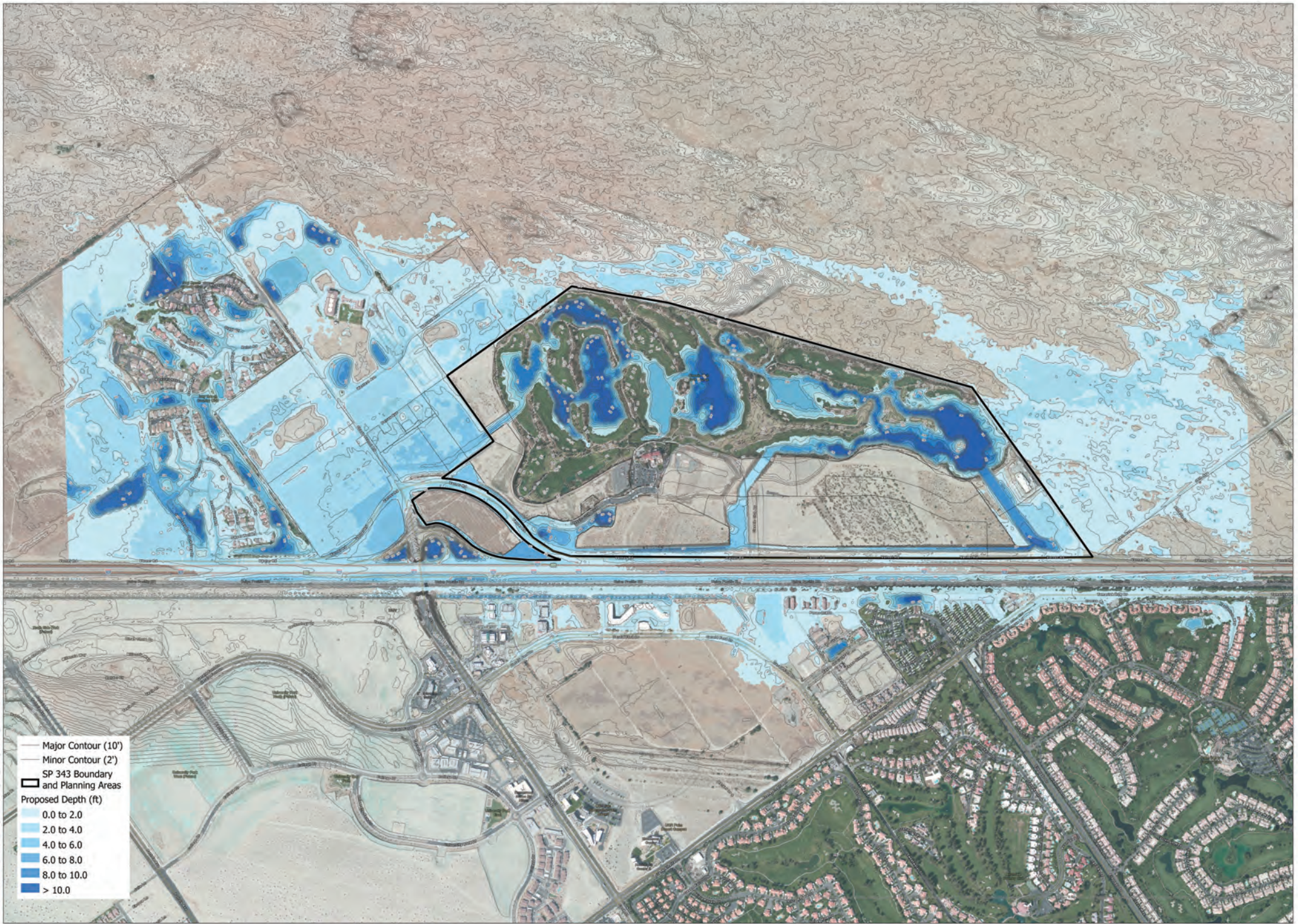
BERGER FOUNDATION Q 100 = 11,600 CFS FLOODPLAIN ROUTING
