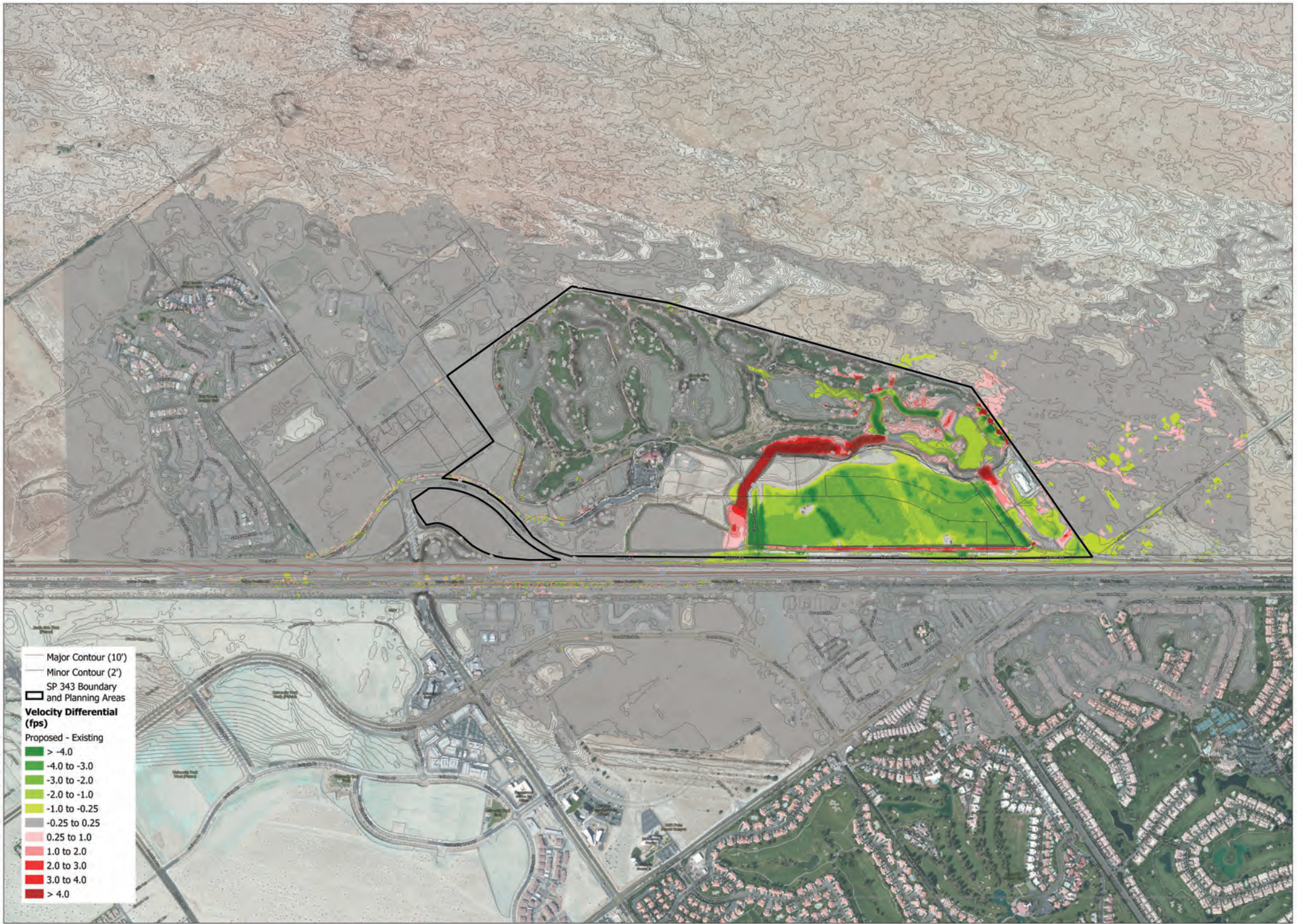
BERGER FOUNDATION Q^{100} = 26,360 CFS FLOODPLAIN ROUTING
