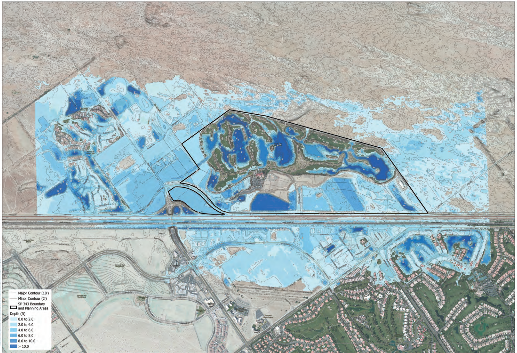
BERGER FOUNDATION Q 100 = 26,360 CFS FLOODPLAIN ROUTING
