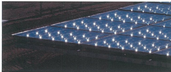
Figure 2: Sun reflection in primary mirror, wind-stowed system, from 10m
