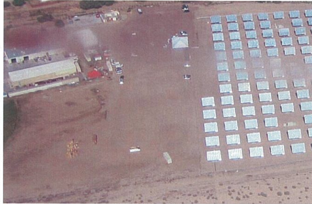
Figure 1: Retro-reflection at Victor Valley College. 400mAGL and 600m distant. Approximately the antisolar point. Systems in operation
