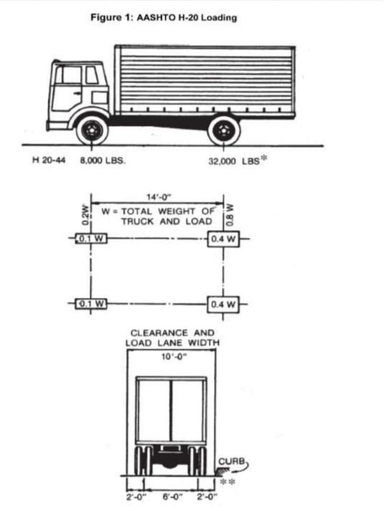
Note: The H loadings consist of a two-axle truck or the corresponding lane loadings as illustrated above. The H loadings are designated "H" followed by a number indicating the gross weight in tons of the standard truck.
