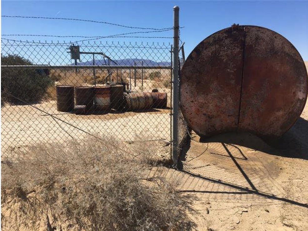
AREA D: View of 12,000-gallon fuel AST and 55-gallon drums with staining and odors near the northern boundary of Area D.
