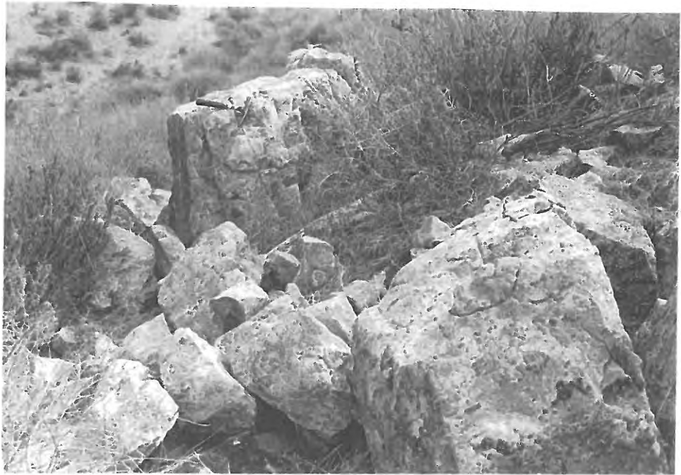
Photo 5 Photograph of igneous-rock outcrop at location HH-5 (Figure 1) showing spacings and orientations of discontinuity planes. Hammer is 0.3 (1 ft) long.
