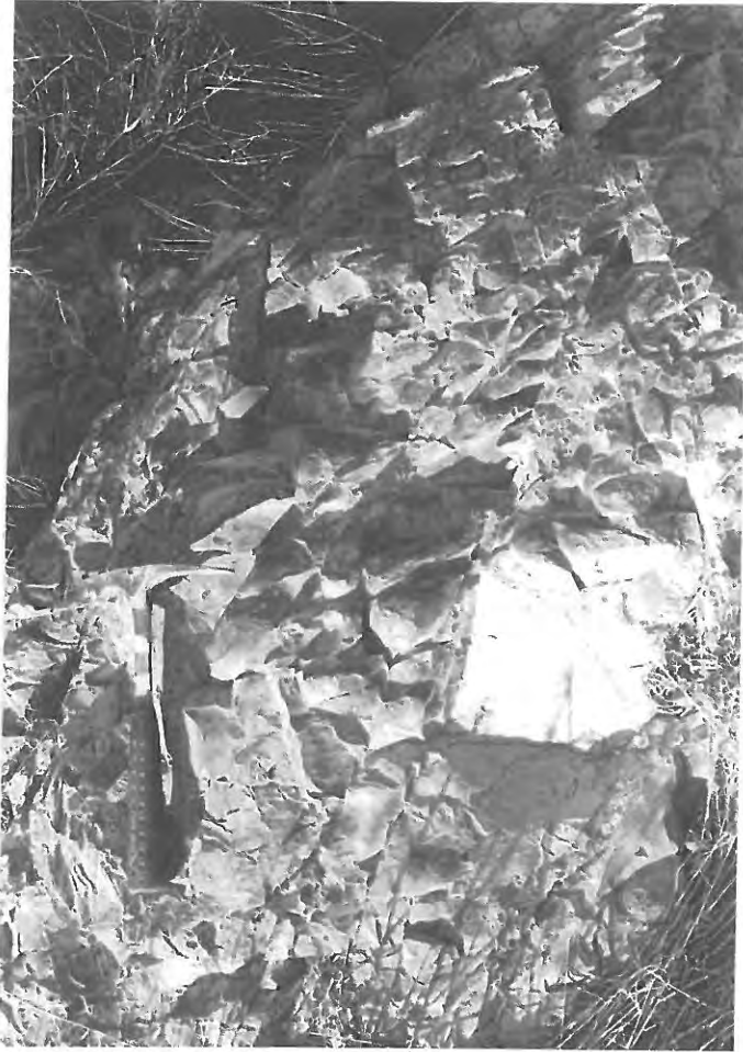
Photo 4 Photograph of conchoidal fracturing and closely spaced discontinuity planes. Conchoidal fracturing is common throughout the metamorphic rock.
