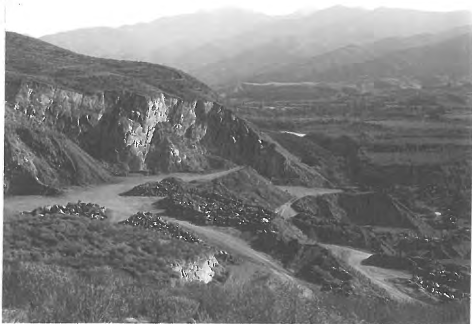
Photo 6 Photograph of Harlow Quarry. Several discontinuity planes are visible within the quarry face. Note the sizes and shapes of the stockpiled rocks that result from the interaction of the discontinuity planes and blasting technique. This would not be possible in the metamorphic rock.
