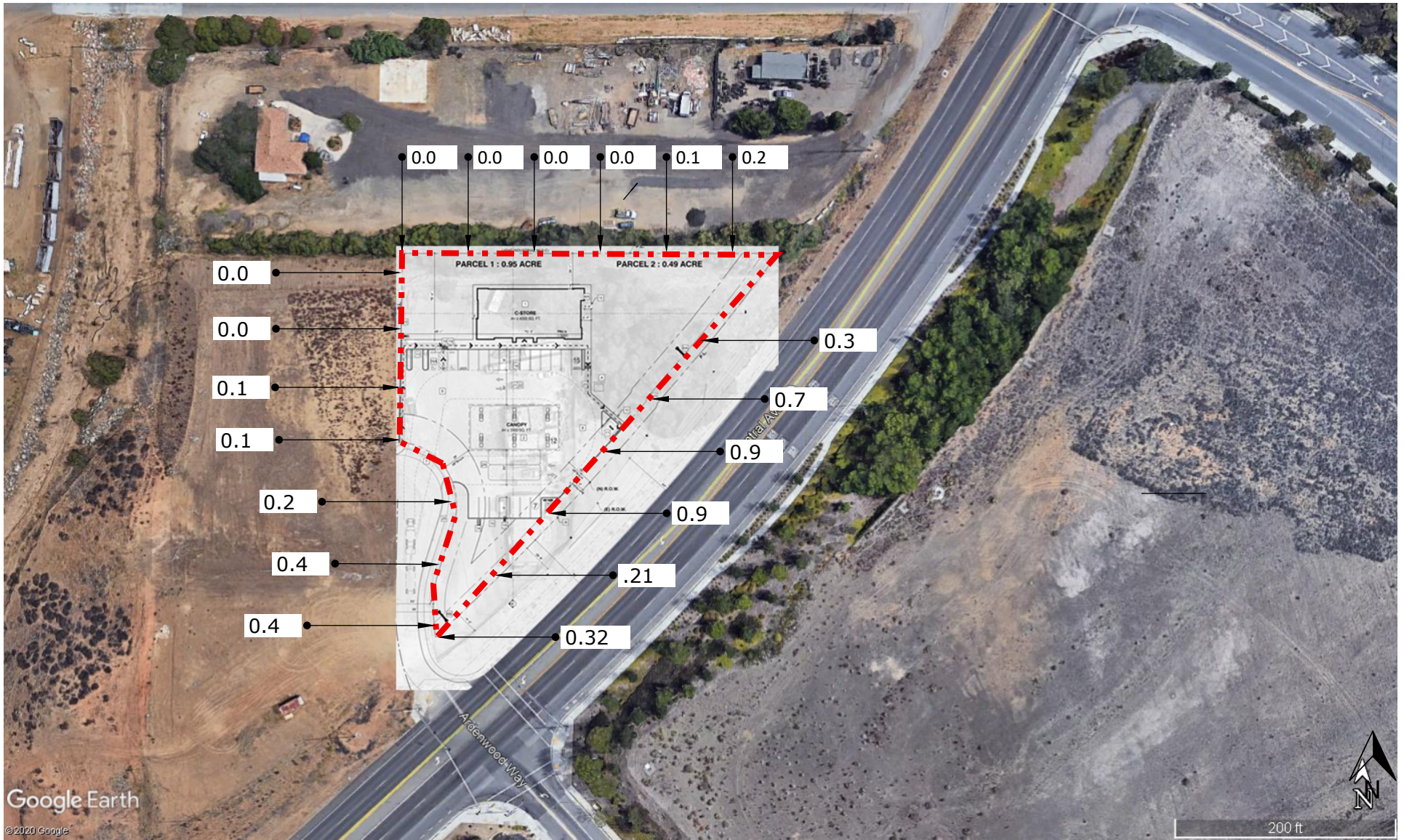
EXISTING LIGHTING LEVELS - GAS STATION & CONVENIENCE STORE 28771 CENTRAL AVE. (74 HWY) LAKE ELSINORE, CA 92532 (MEASUREMENT UNITS = FOOT CANDLE) FOR ILLUSTRATIVE PURPOSES ONLY
