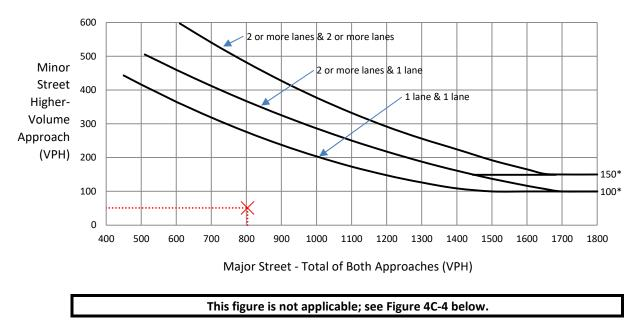
\*Note: 150 vph applies as the lower threshold volume for a minor street approach with two or more lanes and 100 vph applies as the lower threshold volume for a minor street approach with one lane.
